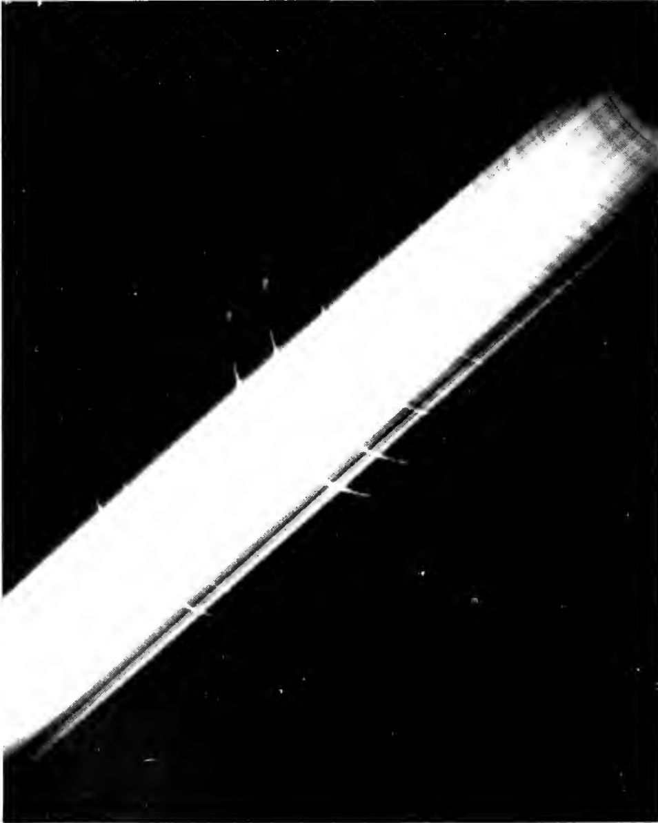
Spectrogram from 60-inch focal length 6-1/2-inch aperture Newtonian telescope with 400 \mu /mm \text{SiO}_2 transmission diffraction grating and spectroscopic analysis No. 1 film. (Newtonian telescope provided by Langley Skywatchers Astronomy Club.)
