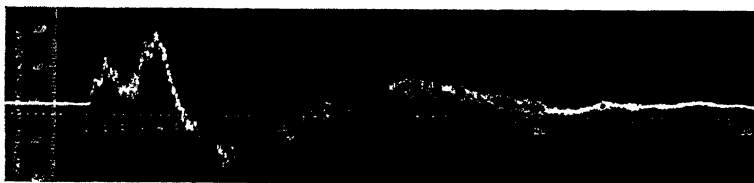
FIG. 43. Phonodeik record of the sound from a 12-inch rifle, distance, 950 feet.
