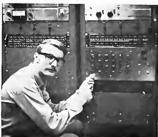
Bob Korzyński points to his program sequencer, which automatically runs six tape machines for over five hours of on-air broadcasting.
