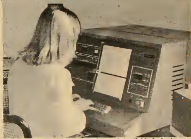
The new CompuGraphic Compuwriter Jr. recently installed in the Southern Accent office to typeset photomechanically all future editions. (Photo by Sharon Webster).
