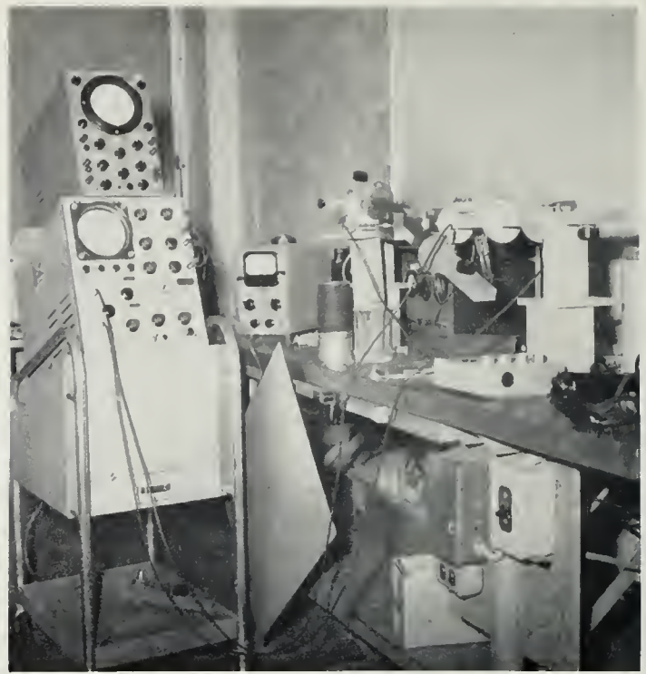
Device here is for the study of plasma resonance at microwave frequencies, a new method of recording molded material.
