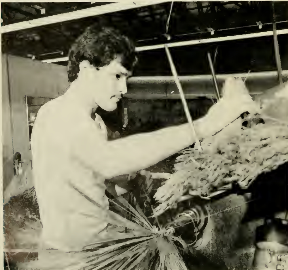
Broom shop employee spins broom corn into the beginnings of a broom.
