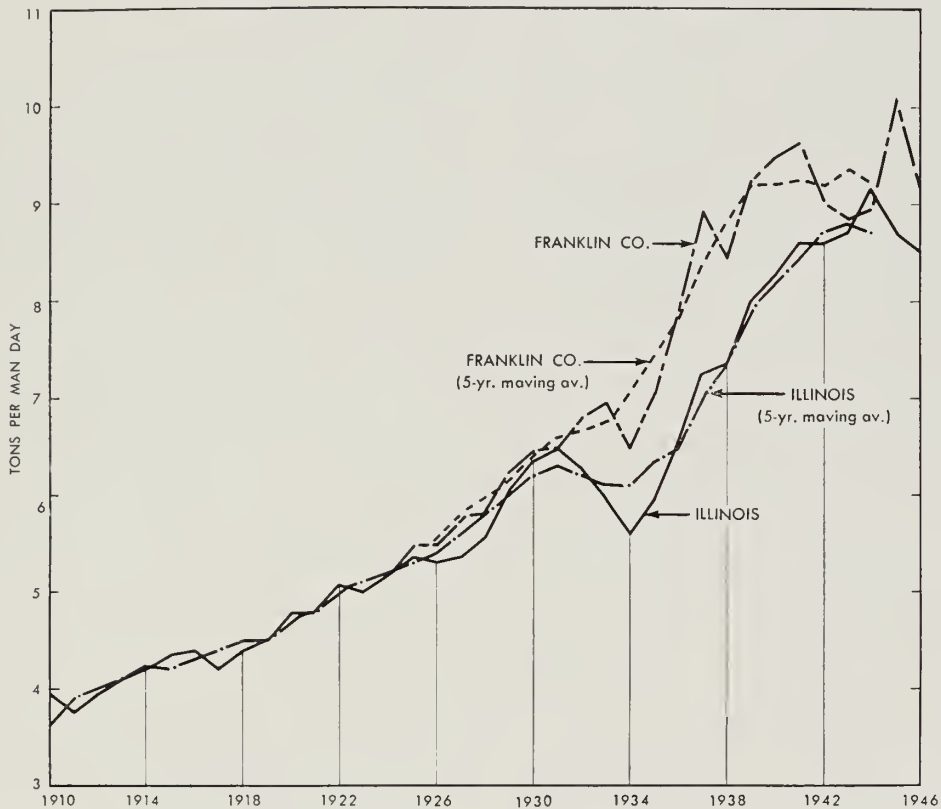
Fig. 35. Tons mined per man day in coal mines in Franklin County and in Illinois, 1908-1946, excluding mines producing less than 1,000 tons annually. ( Minerals Yearbooks , United States Bureau of Mines.)
