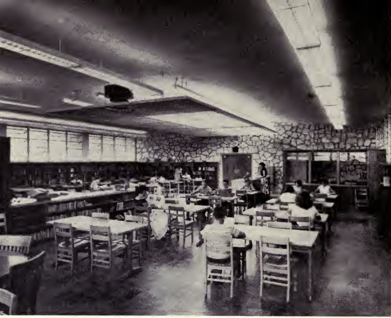
The library at the Madison Junior High School, Miami, has light, acoustical ceiling; modern, indirect lighting; wide glass jalousies, and natural stone wall.
