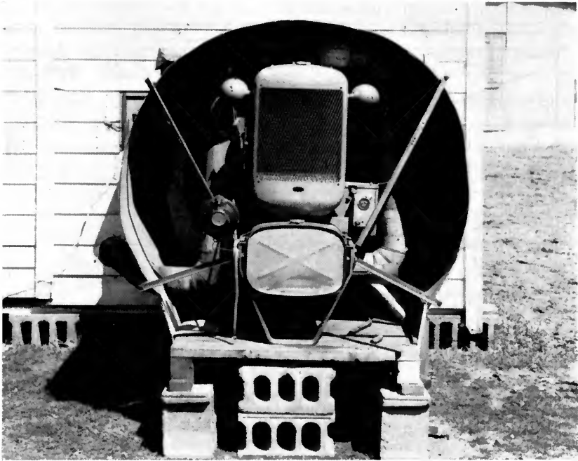
This portable drying unit consisted of a propeller-type fan connected to the drive shaft of a stationary engine. The shield directed inlet air past the engine so as to utilize the waste heat for drying. (See Tests 3 and 4, Table 6.) (Fig. 15)
