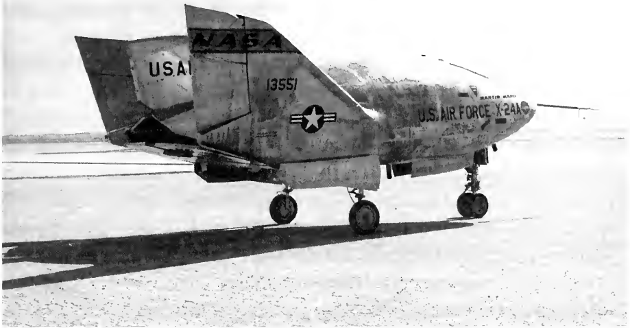
Martin Marietta's X-24A, built for subsonic flight, duplicated the shape of PRIME, which flew at near-orbital velocity. (NASA)(E-18769)
