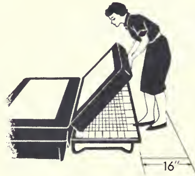
Opening and edging-out space (type tested needed to be moved out from wall to be opened; some do not)
