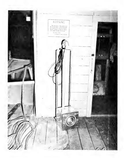
Figure 6.--Watertight aluminum container for submering the electromagnetic transducer.
