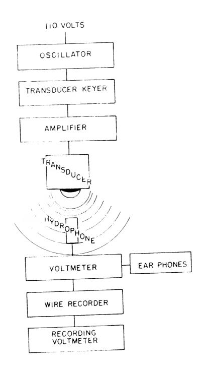
Figure 7. --Block diagram showing electron-unit arrangement.
