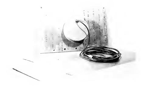
Fi gure 2.--Piezoelectric transducer mounted in the end plate of the experimental tank. The expansion and contraction of the crystal elements, when energized, creates the sound or pressure waves. These waves are transferred into the water through the front of the "can" which is of thin flexible metal. The "can" is filled with castor oil for more efficient expansion and contraction.
