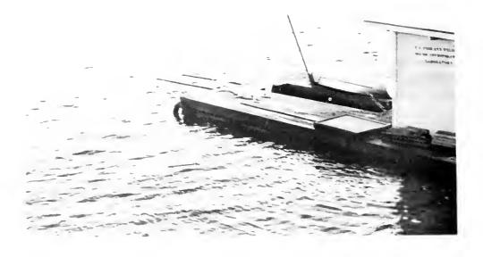
Figure 5.--The floating laboratory on Lake Washington. (Note the rails extending forward, upon which the underwater pen is supported.) The well forward of the cabin allows for easy handling of fish in the pen.
