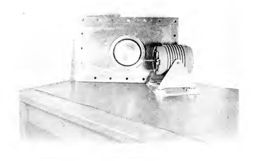
Figure 1.--Electricmagnetic transducer and the end plate from the experimental tank. Note the piston face and the surrounding rubber diaphragm. The piston, when driven by the transducer, created the sound or pressure waves and transferred them into the water. This unit is rated at 100 watts.
