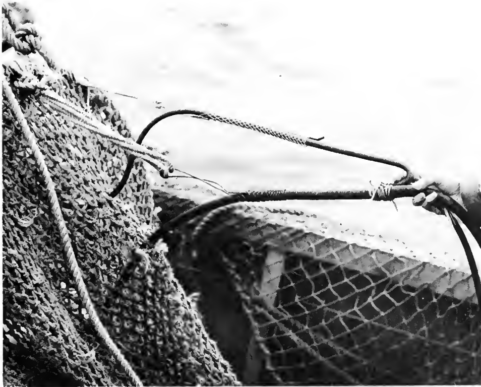
FIGURE 9.--KELLEMS GRIPS ATTACHED TO CAMERA CABLE AND ACCESSORY LIGHTING CABLE.
