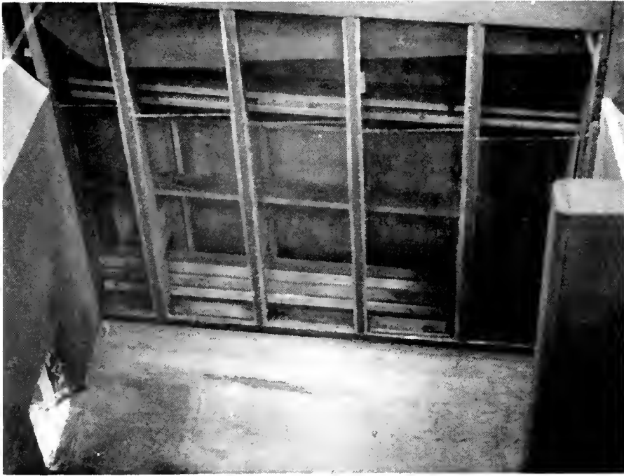
Figure 9.--Interior of the test fishway at pool 59, showing attached observation chamber. Plexiglass wall panels are 3/4-inch thick.
