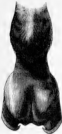
FIG. 545.—Form of Concave Shoe Used by the French for Expanding the Quarters.
