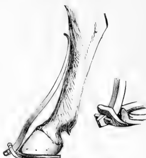
FIG. 926.—Drawing of the Shoe and Bar Used for the Treatment of the Case Referred To.
