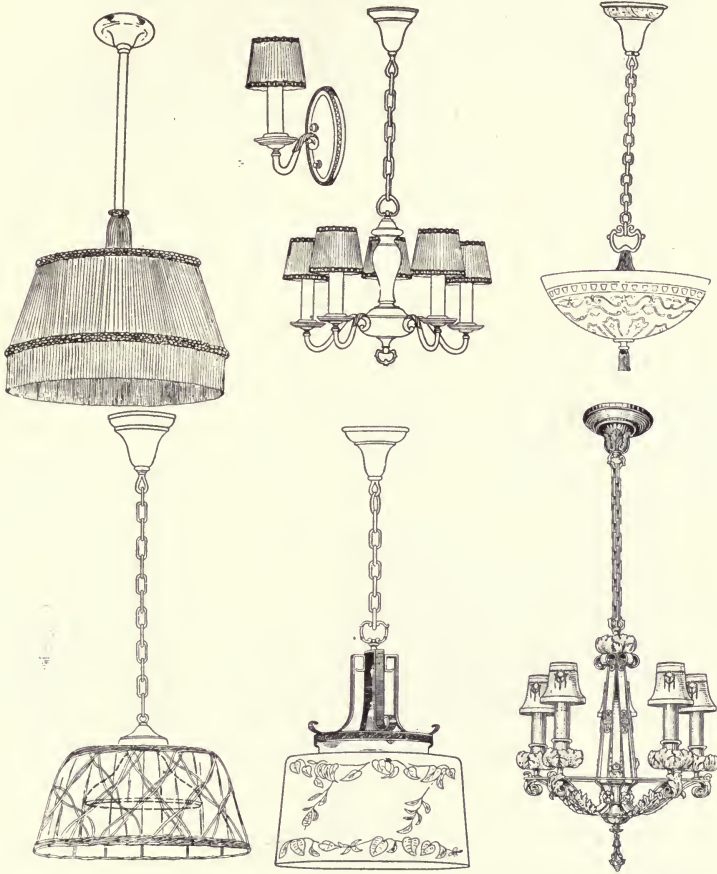
Some Well Designed Dining Room Units. It is of interest to note the tassel at the bottom of the semi-indirect bowl. This conceals half of an attachment plug for use with cooking devices. The wicker dome carries an opalescent reflector indicated by dotted lines
