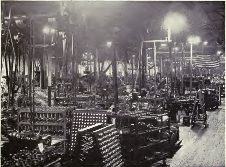
Fig. 1.—Successful Application of Properly Directed and Diffused General Lighting to Interiors of this Nature is Gradually Eliminating the Drop Cord System
