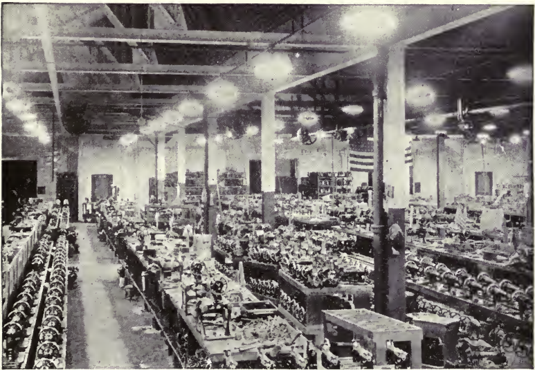
Figs. 7 and 8.—Adjoining rooms in the same factory. The upper figure illustrates a strictly local lighting system of the poorer sort. The lower figure illustrates a lighting system consisting of 150-watt bowl enameled lamps equipped with dome reflectors spaced 10 feet apart; the average illumination is 9 foot-candles.
