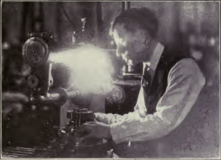
Fig. 9.—Glaring light from unshaded local lamp which is a menace to safety and to vision and is one of the evils which the Lighting Code is expected to eliminate.
