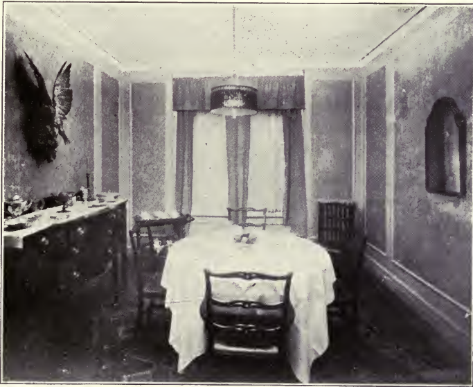
This Night View of the Dining Room illustrates the Even Illumination and Absence of Shadows Characteristic of Semi-indirect Lighting
