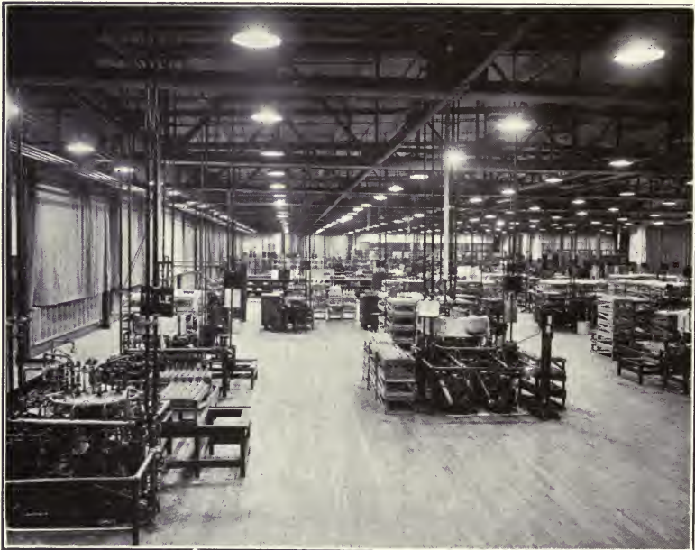
Operations of fine detail may be well lighted by an overhead system. Here the average of 10 Foot-candles is provided by 10' x 10' spacing of 150 and 200 Watt Mazda C Lamps in RLM Reflectors
