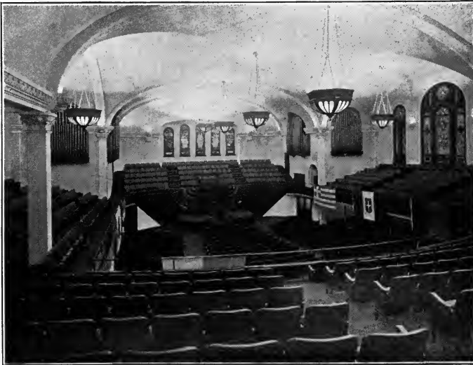
Night View of a Church with Totally Indirect Fixtures of the Luminous Bowl Type. General illumination is furnished by 500-watt MAZDA C lamps in inverted mirrored glass reflectors and 75 watt MAZDA C lamps, in smaller angle units at the capitals
