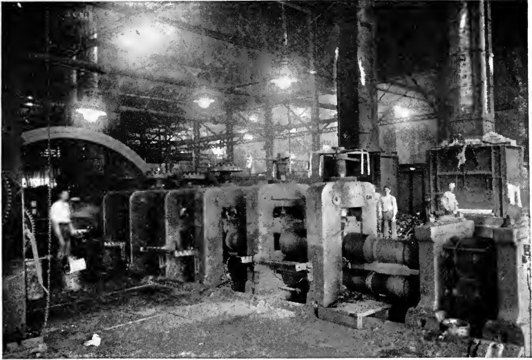
Fig. 13—Lighting of steel rolls. Illumination provided by five mantle inclosed gas arc lamps, equipped with opaque reflectors.
