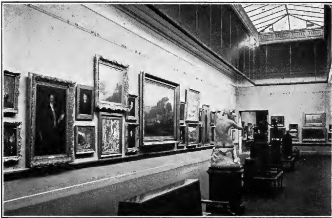
A Night View of a Well Known Painting Gallery Illuminated by 40-watt MAZDA Lamps in a Continuous Rippled Mirrored Glass Reflector.
