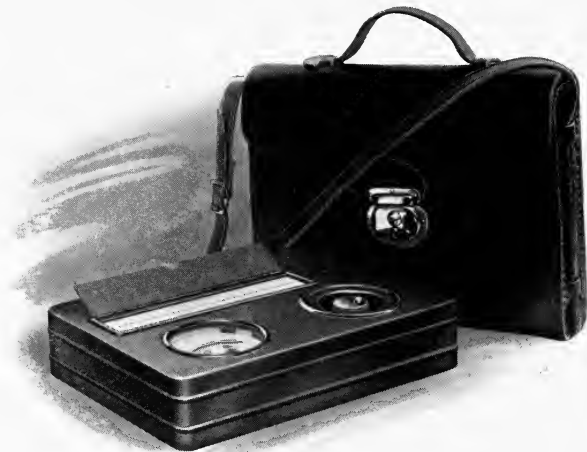
Fig. 3.—The Foot-candle Meter Measures Light at the Work and Reveals the Combined Effect of all Possible Causes of Depreciation
