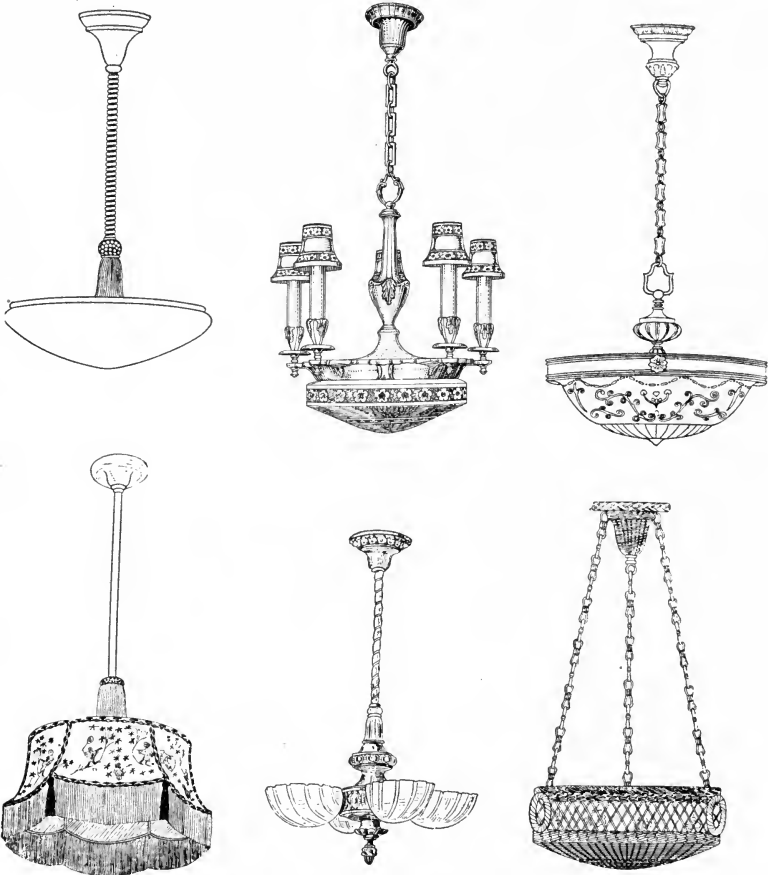
A Few Styles of Direct, Semi-Indirect and Totally Indirect Ceiling Luminaires Suitable for the Living Room Under Various Conditions Glass shades for candle fixtures are now available in very rich and decorative designs
