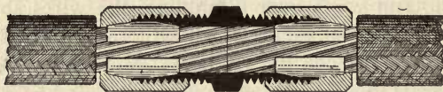
The Dossert Solderless Cable Connector approved for use on stranded wires and cables without the use of solder.
