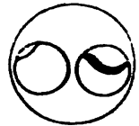
Fig. 296.—Explosion of a Lancashire boiler from the collapse of both of the furnace-tubes.
