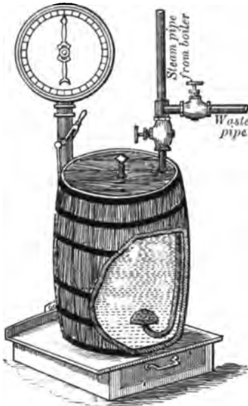
Fig. 270 —Calorimeter for testing the dryness of steam.
