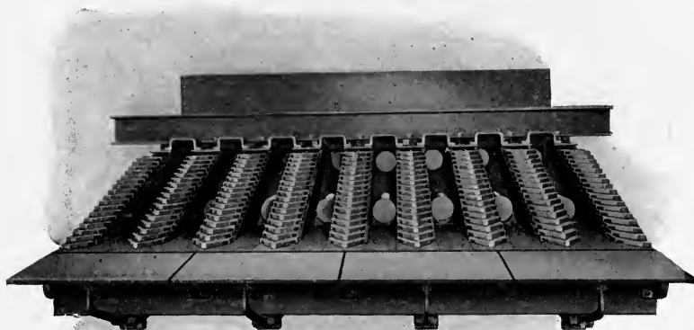
FIG. 81.—Rear view of Taylor gravity underfeed stoker.
