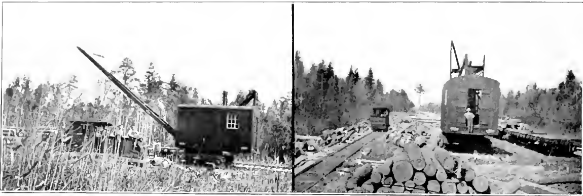
Two views of machine which is used to transfer gum, cypress, pine, and juniper to Norfolk & Southern standard flat cars. Machine located in the center of Dismal Swamp, North Carolina.
