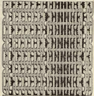
BOTTOM VIEW OF CHAIN SHOWING ROLLERS FOR DRIVING-SPROCKET ENGAGEMENT
