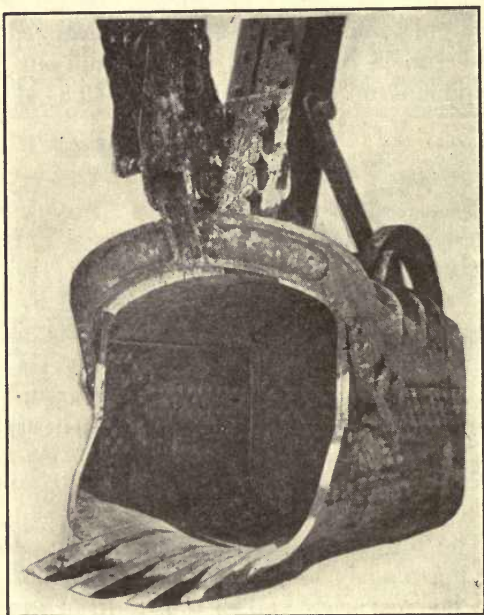
FIG. 5.—Vanderhoef all manganese-steel dipper.
