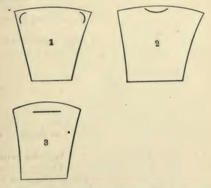
If the axe be cracked as shown in Fig. 1, the corners have been hotter than the middle of the blade; probably by snipping the corners and the middle and comparing the fractures the coarser grain at the corners will tell the tale.
