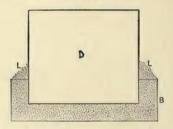
D is the die to be heated; B is an open box about two inches deep and one inch larger each way than the die; L is the burnt leather packed in thoroughly, and as full as the box will hold. The engraved face is down, embedded in the burnt leather, and secure from contact with flame or air.
