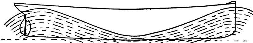
FIG. 30.—Showing tendency to 'sag.'
