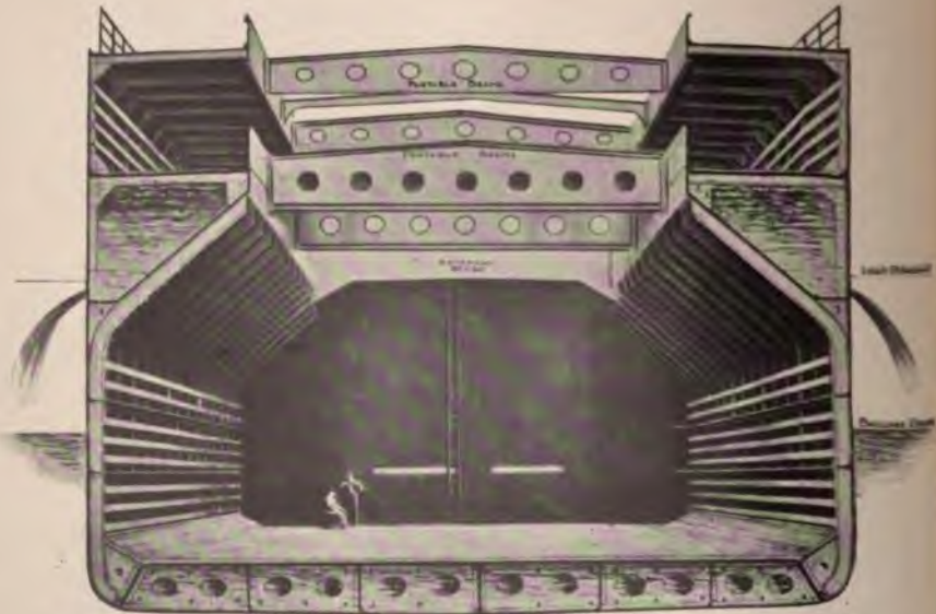
Hold View of Cantilever Framed Ship, Shelter-Deck Type, for Passengers, Cattle, etc.
