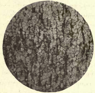
FIG. 105.—0.08 % carbon, hard drawn wire and annealed. Nearly pure ferrite.
