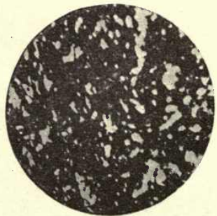
FIG. 87.—Nickel 20%, carbon 0.25%. Savoia.
