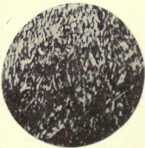
FIG. 86.—Nickel 12%, carbon 0.25%. Savoia.
