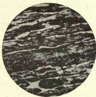
FIG. 112.—Cast steel forged at too low heat, showing distortion of "grain."
