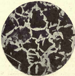
FIG. 108.—0.49 % (overheated) carbon steel. Ferrite (white), pearlite (dark).
