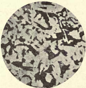
FIG. 17.—0.30% carbon steel. Ferrite (white), pearlite (dark). × 75.
