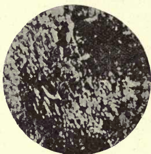
FIG. 91.—Chromium 1.75%, carbon 1.10% overheated.
