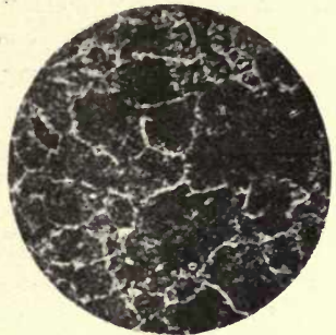
FIG. 68.—After carburizing and quenching direct from box. Coarse structure.
