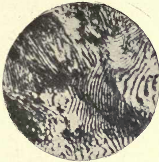
FIG. 16.—0.83% carbon steel, pearlite. × 500
