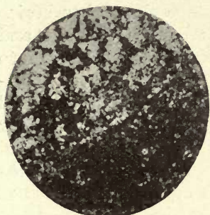
FIG. 76.—Nickel 3.44%, carbon 0.176%, carburized and air cooled.
