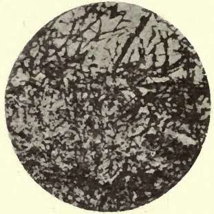
FIG. 83.—Nickel 4.86%, carbon 0.115%, carburized and air cooled.
