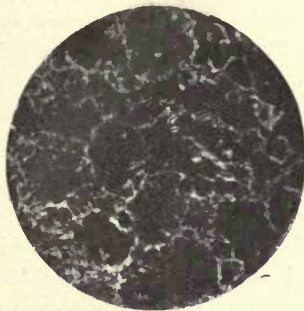
FIG. 69.—Structure after cooling in box and subsequent quenching at 1,200° F.
