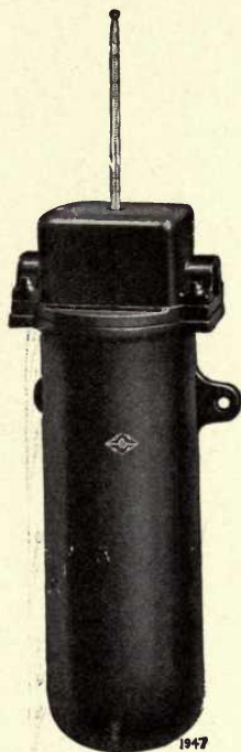
FIG. 58.—Oil-filled vacuum flask for cold junction.
