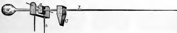
FIG. 182.—Simple Frog's Heart-Lever. a . Fulcrum; L . Glass lever with knob to act as counterpoise; b . To fix the apparatus into the cork of a frog-plate; C . Cork to rest on the heart.
