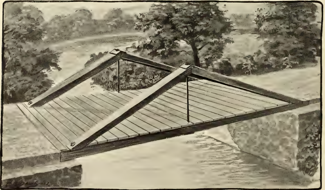
A TRUSS IN THE FORM OF A BROAD "A" TO ADD TO THE STRENGTH.
