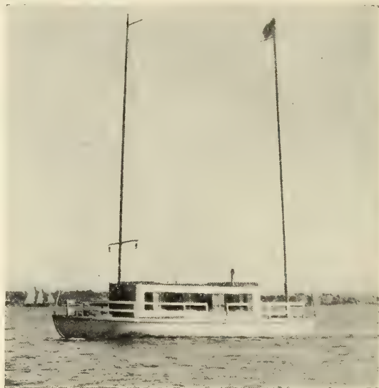
JOHN HAYS HAMMOND, JR.'S HOUSE-BOAT, DIRECTED BY WIRELESS, WHICH PRECEDED HIS WIRELESS TORPEDO-BOAT.
