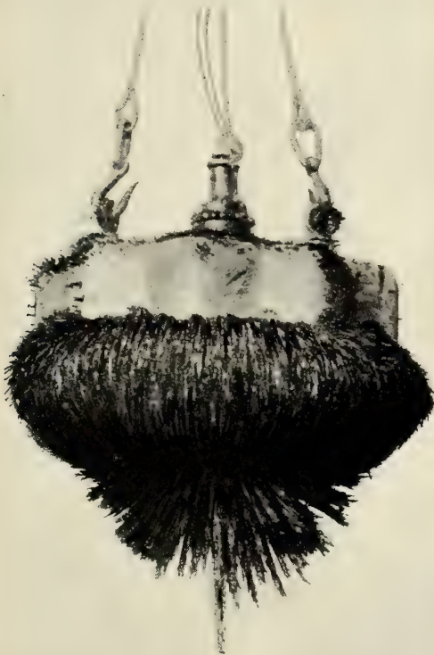
AN ELECTRO-MAGNET LOADED WITH SWEEPINGS FROM A MACHINE-SHOP.
