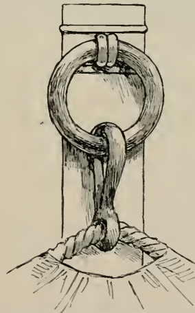
SPRING-CLIP FASTENING COVER TO FRAME.
