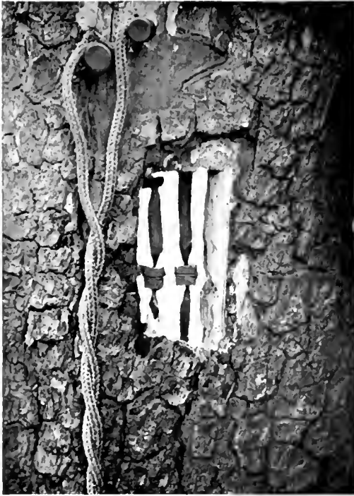
THE "BOX" WITH THE "DOOR" REMOVED, SHOWING THE MICROPHONE AND CONNECTIONS
