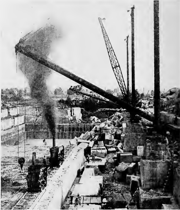
FIG. 4.—Steam channeling machines at work in an Indiana limestone quarry. (Courtesy of Indiana Limestone Company.)
