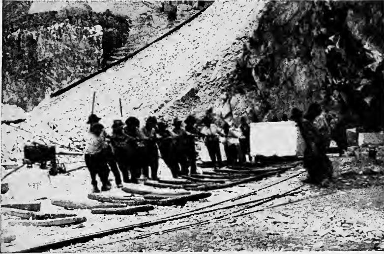
FIG. 64.—Dragging a marble block on greased skids, Carrara, Italy. (Courtesy of J. B. Newsom.)
