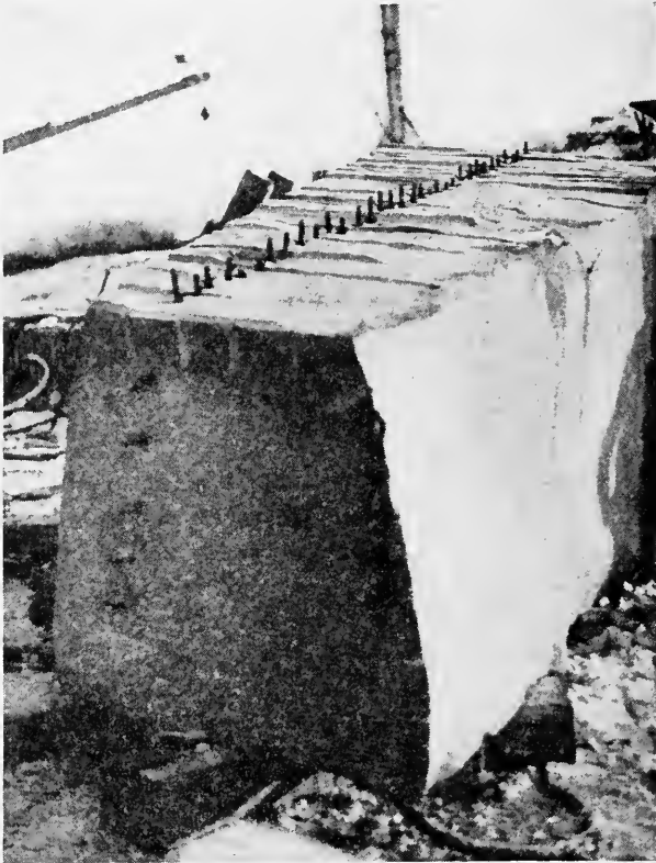
FIG. 26.—Subdivision of a block of granite in a Westerly, R. I., quarry by wedging on top and end. (Photo by the author.)
