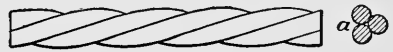
FIG. 43.—Details of steel wire used as wire saw in quarrying, natural size. a , cross section.
