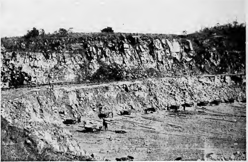
FIG. 73.—A limestone quarry worked in two benches; the stone is loaded by hand.
