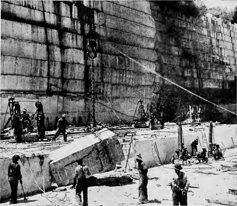
FIG. 36.—A marble quarry showing simultaneous hoisting, channeling and gadding operations. (Courtesy of Georgia Marble Company.)
