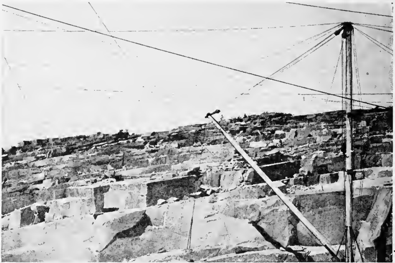
FIG. 24.—A typical New England granite quarry illustrating sheet structure; Stonington, Me.
