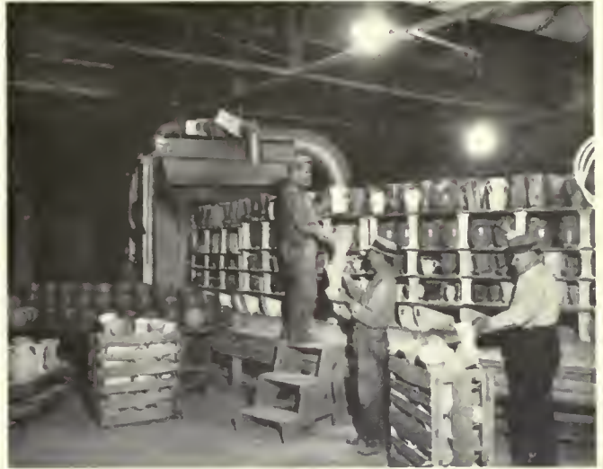
Unloading Pottery from a Tunnel Kiln
