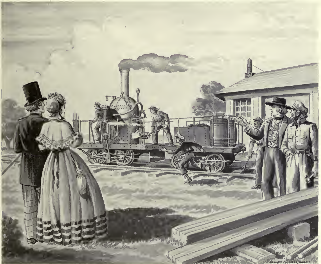
"The York," with Phineas Davis as engineer, chugged off in fine style, at a speed of thirty miles per hour, on its test run before the directors and engineers of the Baltimore and Ohio Railroad, August 4, 1832.
