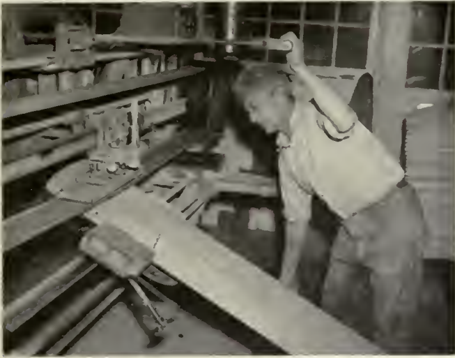
A specially designed belt sander contributes to the ultimate high quality finish, characteristic of the York product.
