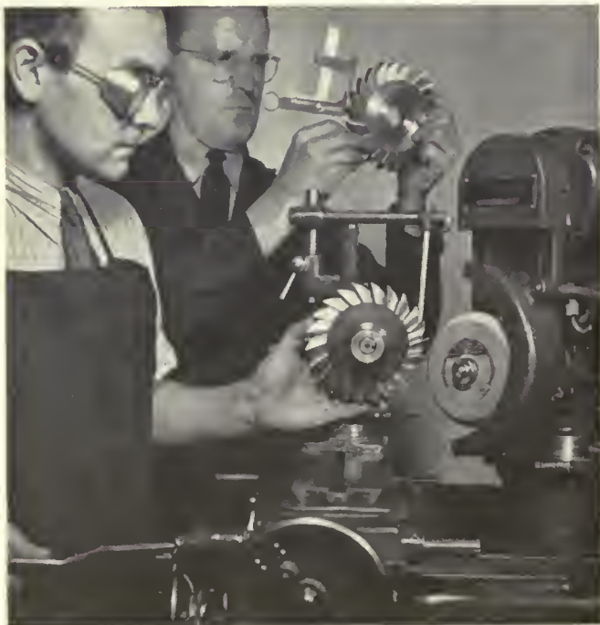
Making precision cutting tools for milling machines at the Atrius Wanner Vocational School.
