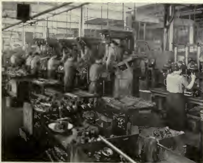
Torpedo parts for steam torpedoes—an extremely close precision job machined to exacting tolerances.
