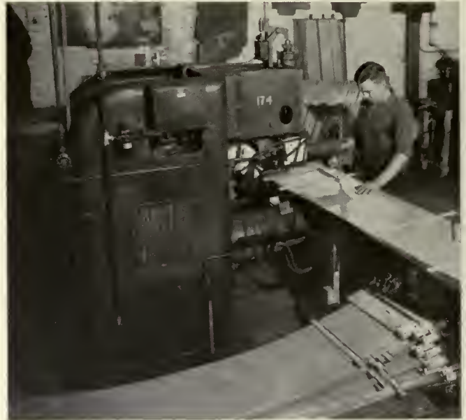
One of a battery of spot welders in operation. Many types of welding units are employed to perform specific operations.
