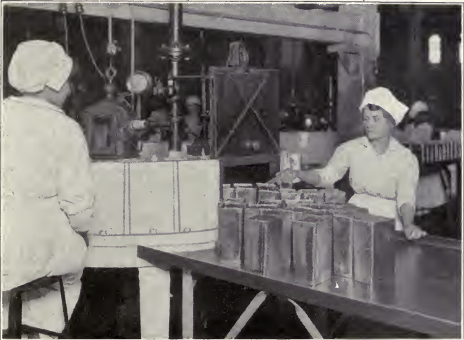
Corned-beef tins coming from the vacuum-sealing machine. The filled tins are automatically conveyed to the sealing machine
