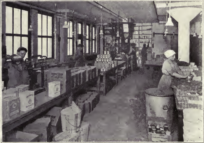
Packing spices. The modern airtight packages into which ground spices are sealed preserve their flavor and fragrance
