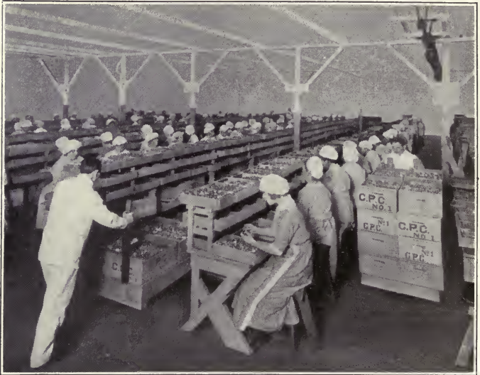
FIG. 37. Assorting and stemming a big shipment of cherries in a canning plant
