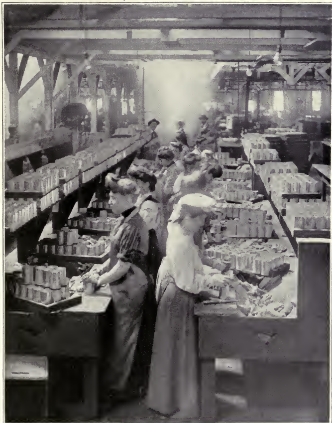
Packing salmon in tins. This slow method of packing by hand has been replaced in most factories by machinery
