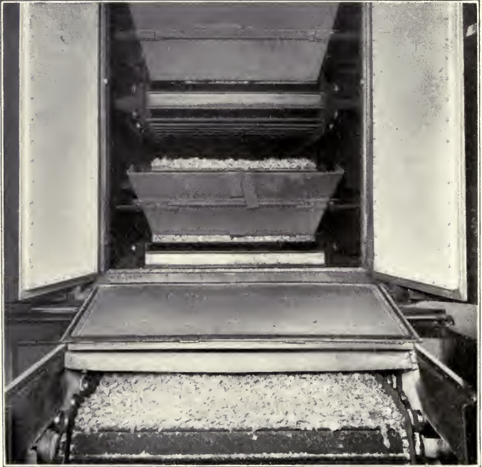
Toasting oven used in the manufacture of ready-to-eat breakfast foods. Toasting not only makes the food crispier but adds color and flavor
