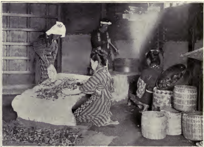
Steaming tea in Japan. The first step in the sterilizing of tea
