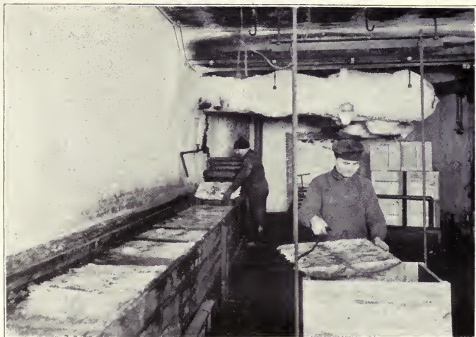
In the freezing room of a wholesale fish market. Taking the fish from the glazing tank
