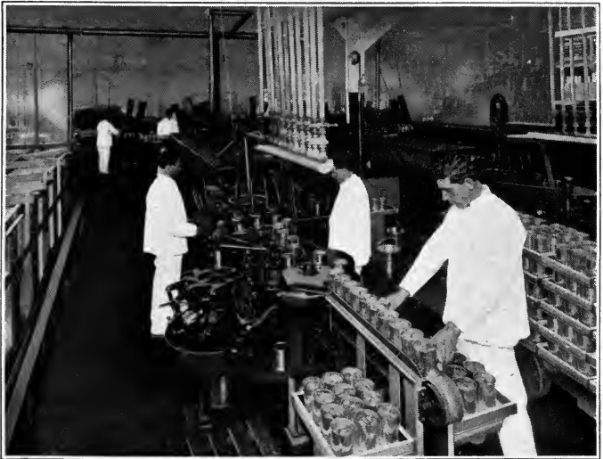
After the cans are filled with boiling hot fruit or vegetables they are carried on a belt to the compressed air "capper," which automatically clamps on the lids
