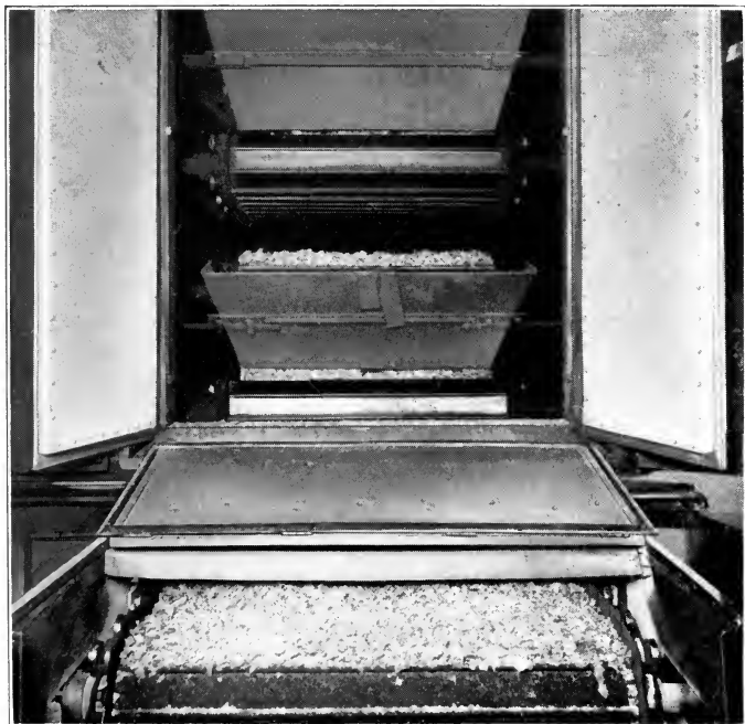
Toasting oven used in the manufacture of ready-to-eat breakfast foods. Toasting not only makes the food crisp but adds color and flavor
