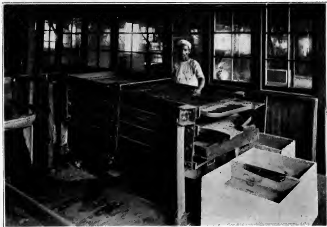
Sorting tea by mechanical sifters into grades and qualities known as pekoe, orange pekoe, pekoe souchong, and souchong
