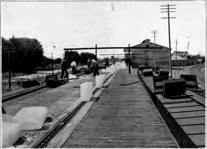
Icing a "passenger express refrigerator" car with an automatic chain ice conveyor
