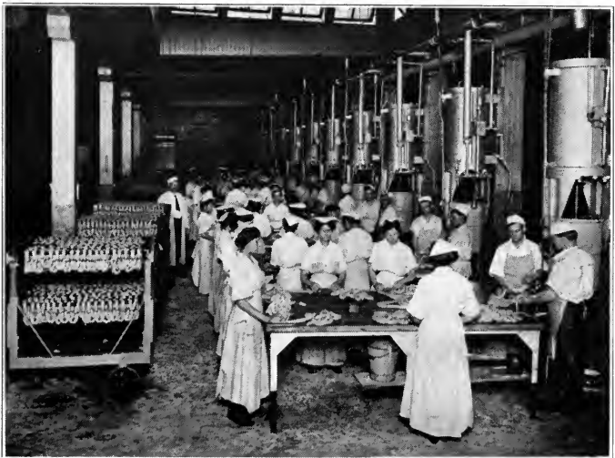
In a sausage factory. Here pork changed into sausage is being stuffed into "casings" and made ready for marketing
