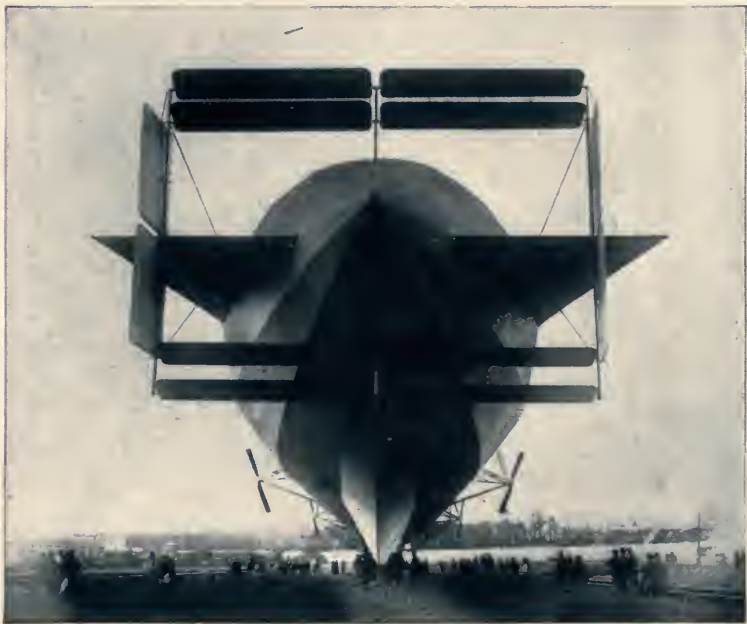
A stern view of the French dirigible "Speiss," showing its elevators and rudders. This airship somewhat resembles a German Zeppelin
