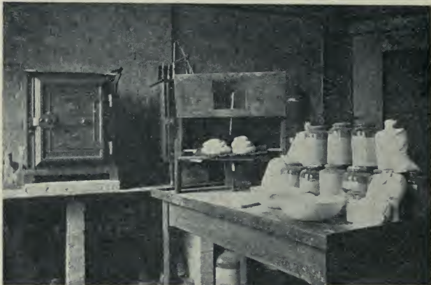
Fig. 16. Apparatus arranged for a baking test. Four loaves which have just been scaled and moulded are seen in an incubator where they are left to rise or prove before being transferred to the oven
