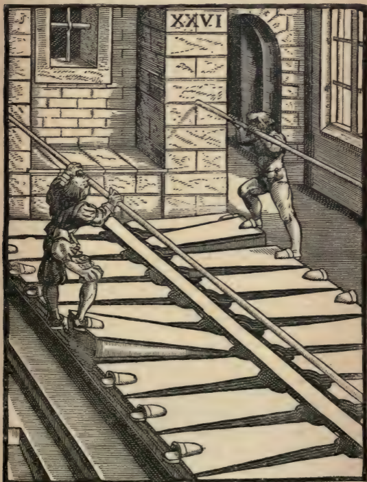
German Organ Bellows of the Sixteenth Century ; showing the feet-holes for the working of two bellows alternately by the treader or blower.
