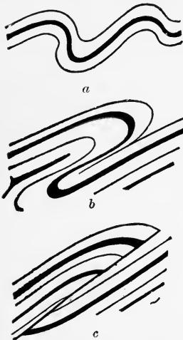
FIG. 92.—PROCESS OF CONVERSION OF A FOLD [a] THROUGH AN OVERFOLD [b] INTO AN OVERTHRUST FAULT [c].
