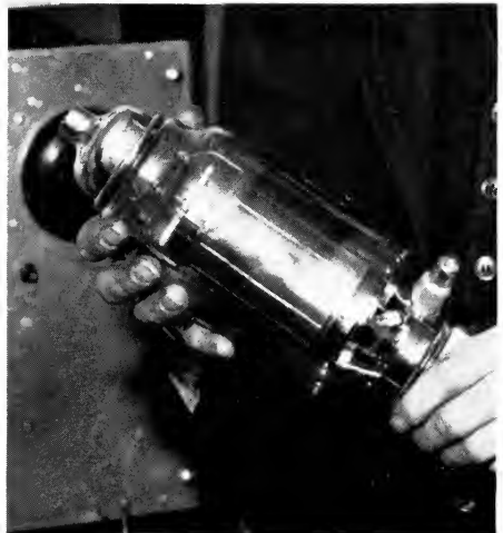
Recent design of the multipactor tube
