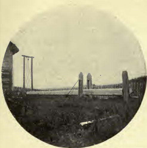
Fur press in use at Fort Good Hope, at the extreme north of Hudson's Bay Company's territory.
