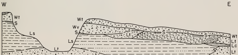
FIG. 2.—Diagram showing facies relations of Lemont drift in gravel pit at Worth, Ill. (locality 8). Wt, Tinley till; Wv, Valparaiso till; S, Sangamon soil on Lemont drift; Lt, Lemont till; Lg, Lemont gravel; Lc, Lemont clay; Ls, Lemont silt with some sand. Vertical interval about 30 feet; horizontal distance about 800 feet.
