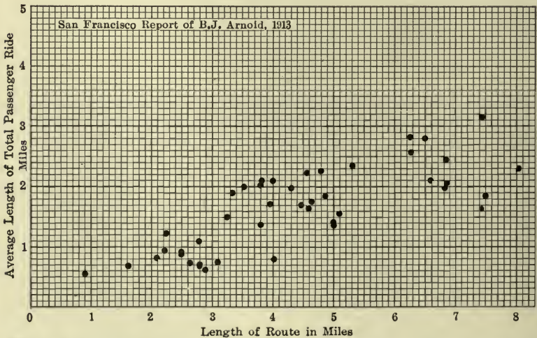
FIG. 24.—Relation between average length of passenger ride and length of line or route.
