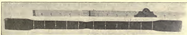
FIG. 28.—Elongation of tension test piece.
