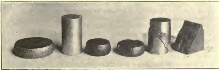
Aluminium, after and before. Mild steel. Wrought iron. Cast iron.
