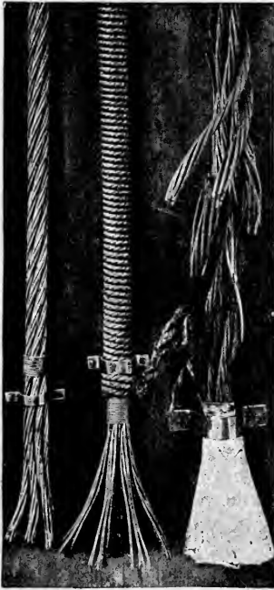
FIG. 244.—Method of capping wire ropes.
