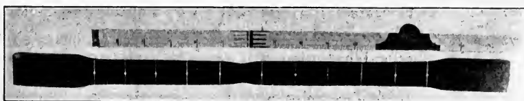
FIG. 28.—Elongation of tension test piece.
