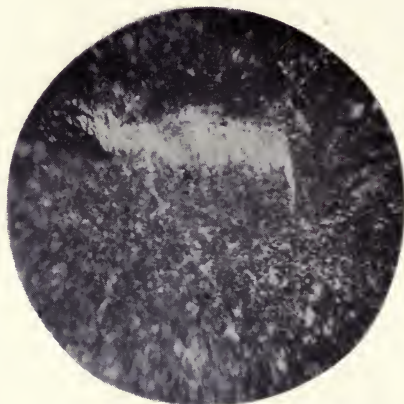
Fig. 1.—Flint clay, Mt. Savage, Md., between crossed nicols. Shows development presumably by hydro-micas along a slip plane \times 160 .
