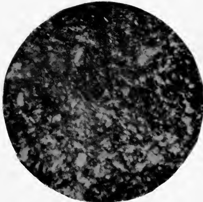
Fig. 2.—Soft clay, Woodland, Pa., between crossed nicols. Shows coarse mat of plates with scattered muscovite grains or flakes \times 60 .
