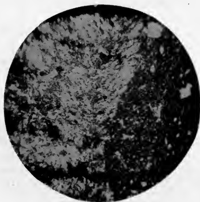
Fig. 2.—Section from Strasburg, O. Shows line of contact, the darker portion representing flint clay and the lighter portion the semi-flint clay with high development of the hydro-micas \times 160 .
