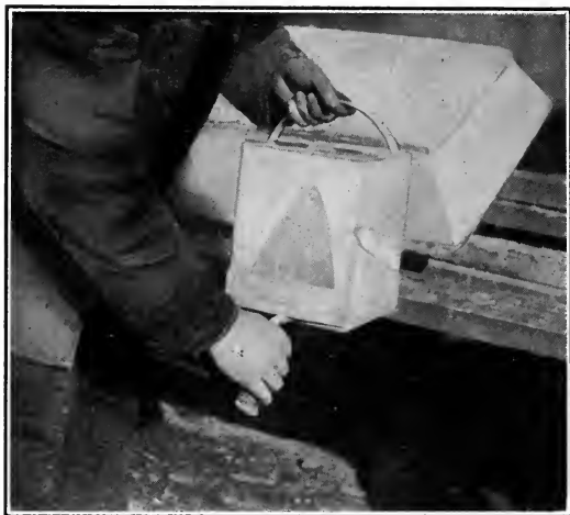
Fig. 19.—The Fountain Trowel for conveying and spreading mortar for 21 brick. The regular trowel forms a temporary handle for lifting and guiding it.
