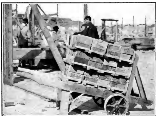
Fig. 21.—Trucket for storing reserve packs stacked up 2 ft. high, to save stooping when it is being unloaded.
