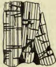
Fig. 6. Pyrrhotite veinlets cutting hornblende. Flaad mine, Evje, Norway. (x 50.) (After Vogt, loc. cit. , p. 139.)
