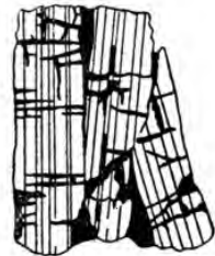
Fig. 6. Pyrrhotite veinlets cutting hornblende. Flaad mine, Evje, Norway. (x 50.) (After Vogt, loc. cit. , p. 139.)
